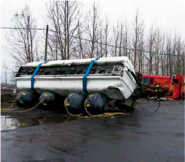
Efficient lifting of overturned vehicles.
